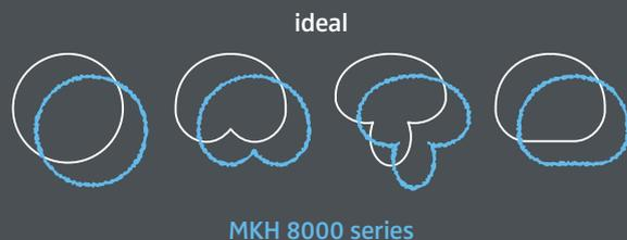
**Accurate directional patterns:** All directional patterns have been carefully designed for minimal deviation from the ideal patterns over the entire frequency range. The unique technical design characteristics of the MKH symmetrical microphone series means that the designer no longer has to make compromises between frequency response, polar pattern and low noise—now he can have it all: wide frequency response, ultra low noise and a polar response close to the theoretical ideal.
